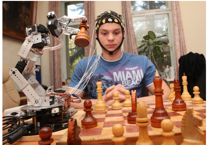
Fig. 1. An example of playing an unmodified game using a P300 BCI (here, using a BCI-controlled 6-DOF robot arm) for testing purposes.
