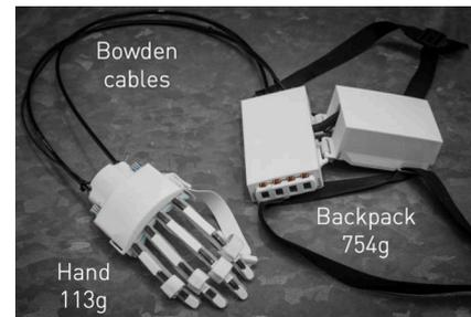
**Figure 1: 3D-printed soft hand exoskeleton. Motors, electronics and battery are placed in the backpack.**
